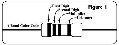
silver indicating 10 %, gold indicating 5 %, and red indicating 2 %. If it is difficult to read the colors, the resistance should be checked with a multimeter.
