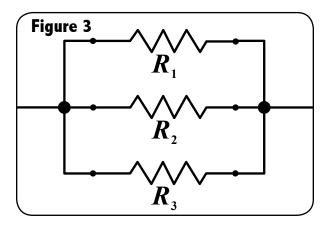
The sum of a set of parallel resistors is the reciprocal of the sum of the reciprocals of the resistor values:
